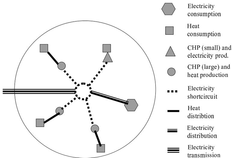
Figure 1: Connections between generation, consumption, distribution and transmission in one region, with one electrical transmission connection to another region.
